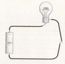
Notice the two loose ends of the wires at the right of the diagram. That's our switch. Assuming that the batteries are good and the bulb isn't burned out, touching these loose ends together will turn on the light.
